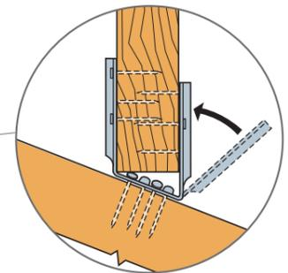
Truss connection to top chord of truss
