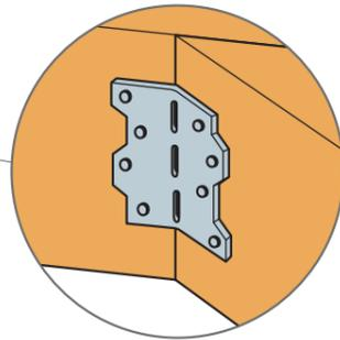
Rafter fixing to corner trusses
