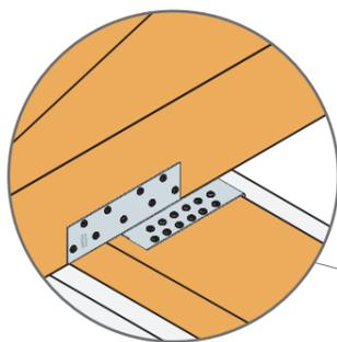
Truss fixing to wall plate
