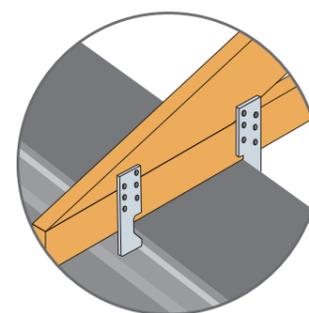
Truss fixing to a steel I-beam
