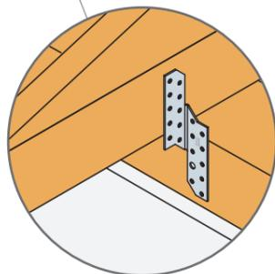
Truss fixing to wall plate
