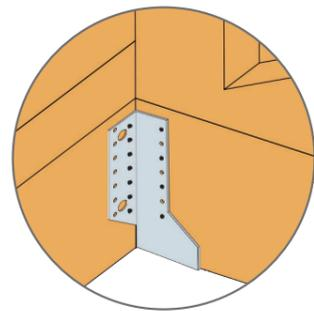
Truss to truss face fixing
