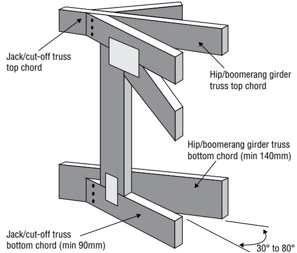
2. With the short leg against the girder, align the Boomerang Connector with the incoming truss with a 6mm offset above bottom edge of the bottom chord. If necessary, bend the Boomerang Connector to the skew angle before aligning.
