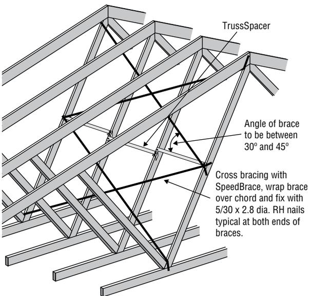
The TrussSpacer can also be used as permanent lateral bracing for webs in standard roof trusses for domestic constructions. The TrussSpacer can be used as a web tie where truss designs require bracing to be applied to webs for the following conditions.
