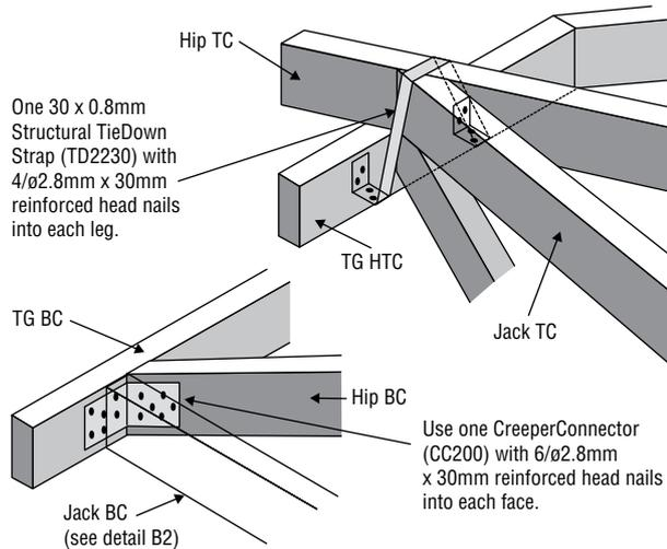
**Detail B2 - Jack Truss to Truncated Girder Truss**
