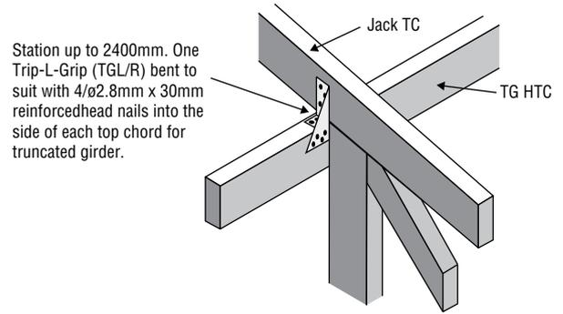
**Detail C2 - Intersection of Jack and Hip Truss to Truncated Standard Truss**
