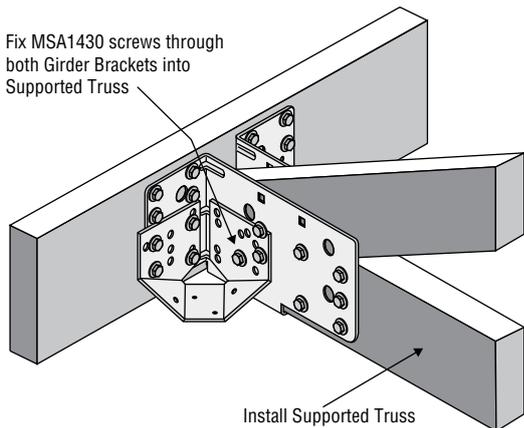
4. Install supported truss on FastFit Girder Bracket and position it hard against the girder truss to ensure all trusses are plumb.
