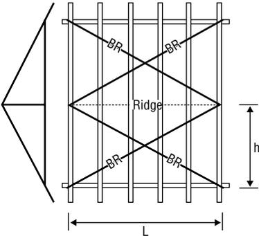
**3. Long Roofs.** Where the roof length "L" is long compared to the half span "h" of the roof trusses and would result in a brace angle less than 30°, two or more crossed bracing bays are required each side of the ridge to ensure the brace angle is between 30° and 45° as shown.
