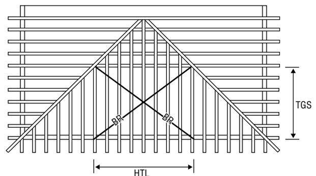
3. Where the horizontal top chord length (HTL) is longer than 1.5 times the truncated girder station (TGS).
