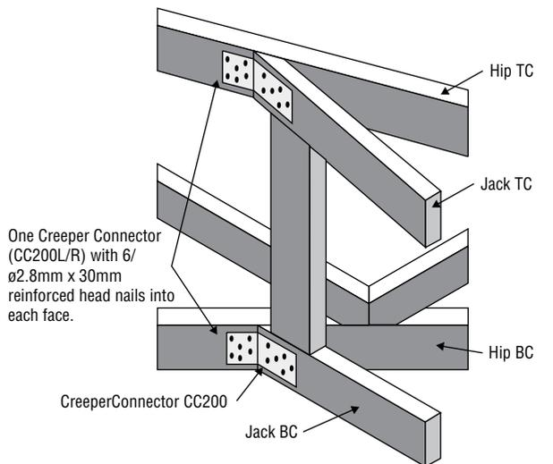
**Detail F2 - Jack Truss to Hip Truss (maximum jack station 3000mm)**
