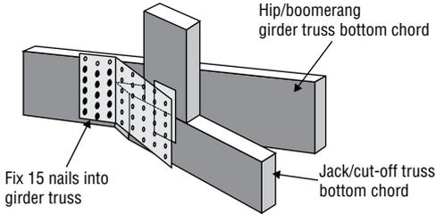
4. Wrap the Boomerang Connector around the mitre cut face and fix 3 nails into the mitre fold.
