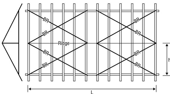
Where the roof requires double SpeedBrace, fix as shown above.
