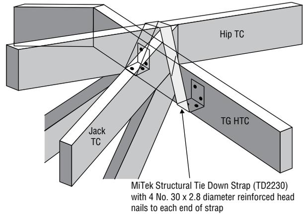
**Detail B. Fixing of Hip Truss to Truncated Girder Truss**
