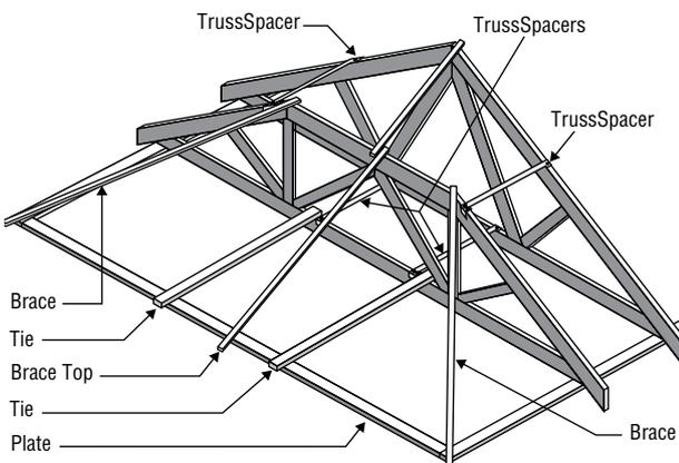
Each successive truss should be spaced using TrussSpacers. TrussSpacers are recommended in lieu of gauging rod or timber ties, as these can be fixed to the trusses prior to lifting trusses on to top plates.
