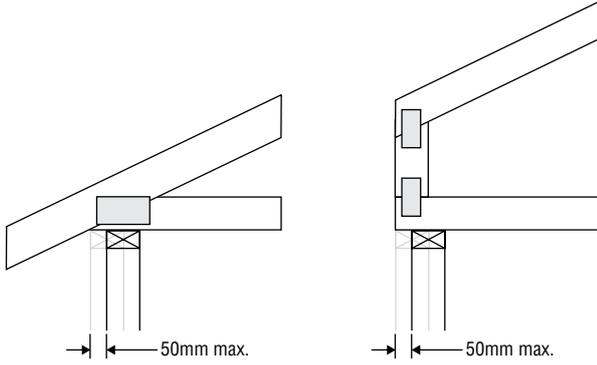
When truss heel or end of cut-off truss is shorter than wall support, the maximum tolerance is half the wall thickness, up to 50mm. Check bearing strength where bearing area is reduced.
