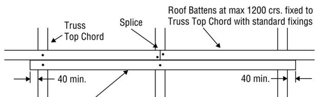
Bridging Batten same size and grade as the batten fixed to Truss Top Chord using 1/14g type 17 screw with minimum 45mm penetration into top truss chord or equivalent
