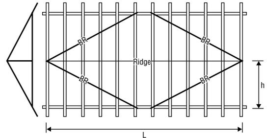
4. **Very Long Roof** – where the roof length "L" is more than 4 times the half span "h" of the roof truss.
