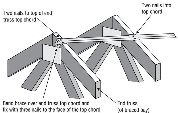
4. To splice SpeedBrace, overlap or wrap around over one truss and fix with three nails. Splice to be located at least 2500mm from heel end fixing, measured along brace.
