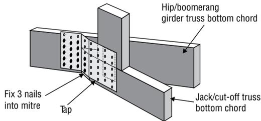
5. Further wrap the connector flush with the jack/cut-off truss. Then fix another 15 nails into the vertical web and bottom chord of the jack/cutoff truss.
