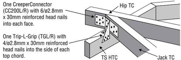
**Detail D2 - Extended Jack or Hip Truss to top chord of Truncated Standard Trusses**
