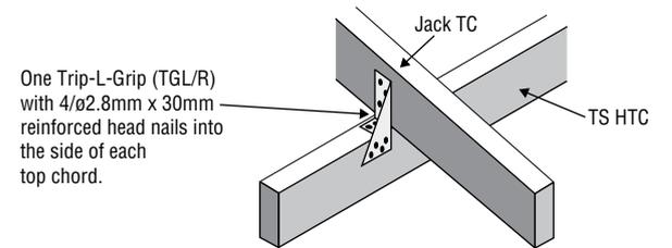
**Detail E2 - Jack Truss to Hip Truss (maximum jack station 2400mm)**
