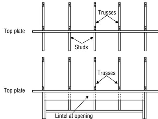
**Top plate strengthening may be required where trusses do not coincide with studs.**
