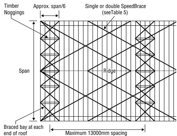
b) For jack trusses or rafters, use single SpeedBrace in an 'X' configuration and the angle of SpeedBrace to end wall should be between 30° and 45°.
