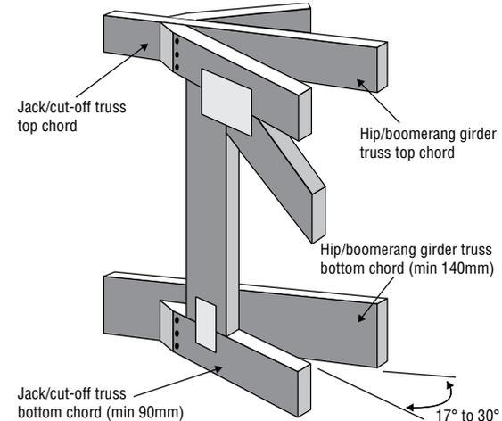
2. With the short leg against the girder, position the bend line along the tip of the double mitre. Offset 6mm above the bottom of the bottom chords.
