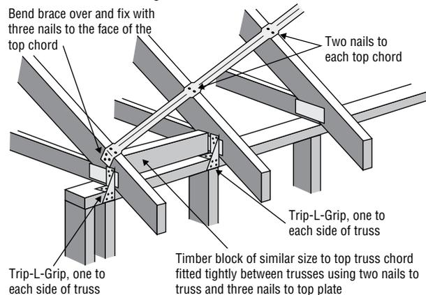
Where the standard trusses are supported by a girder truss or a beam rather than a wall top plate, fix SpeedBrace at truss heel as shown following.
