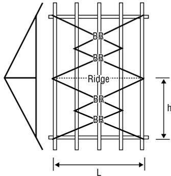
**2. Short Roofs.** Where the roof length "L" is of length to give a brace angle between 30° and 45° then only one bay of bracing is required each side of the ridge line as shown
