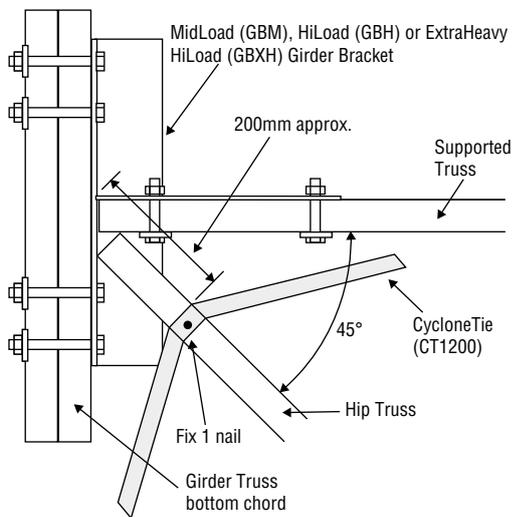
2. Bend one leg under the bottom chord of the incoming girder and the other under the supporting girder. Tap slightly to make a tight bend then wrap them under the chords and fix with 4 nails as shown in diagram below.
