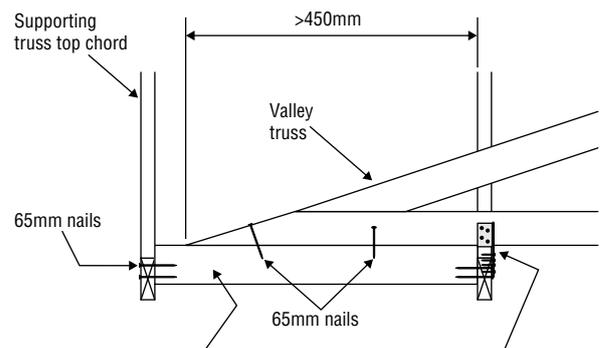
Block infill (minimum 75 x 35) to where the saddle truss is cantilevered more than 450mm or where the saddle truss is not supported by two truss top chords, fixed to the saddle truss bottom chord with 2/65mm nails, and to each end to supporting truss top chord with 2/65mm nails
