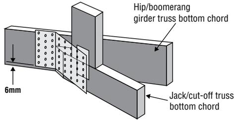
3. Fix 15 nails into the hip/boomerang girder bottom chord.
