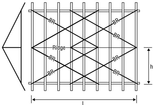
**4. Very Long Roofs.** As for long roofs, except continue bracing for length of building such that each truss is crossed with at least four braces.
