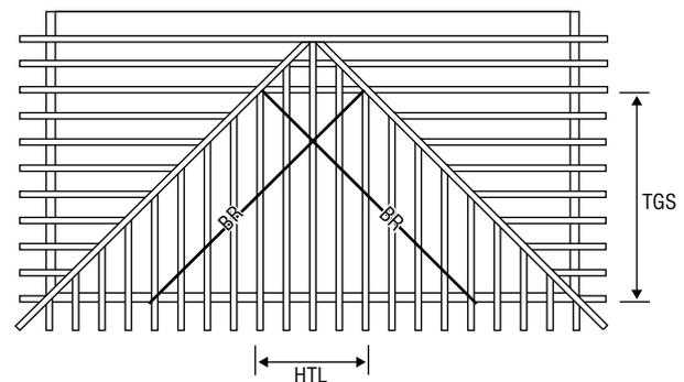
2. Where the horizontal top chord length (HTL) is 1 to 1.5 times the truncated girder station (TGS).
