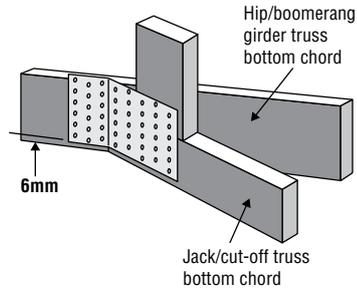
3. Ensure the connector is flush with the chord surface and fix 15 nails into the hip/boomerang girder bottom chord and 15 nails into vertical web and bottom chord of the jack/cut-off truss.
